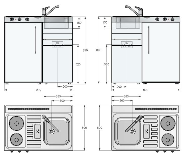
Fridge - 13 amp 3 pin plug 136 kWh/annum Hotplates - 13 amp 3 pin plug 2.2kW Ceramic - 13 amp 3 pin plug 3kW Induction - 3.5kW Fused spur (13 amp 3 pin plug available on request)
